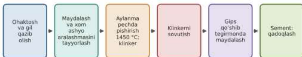
22-rasm. Portlandsement ishlab chiqarishning texnologik sxemasi
