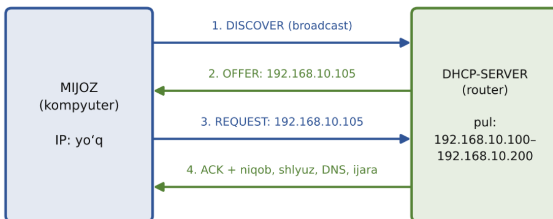
2-rasm. DHCP orqali IP-manzil olish jarayoni (DORA)
