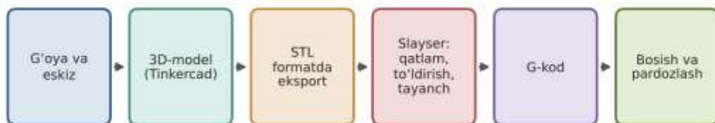
29-rasm. 3D bosma jarayonining bosqichlari
