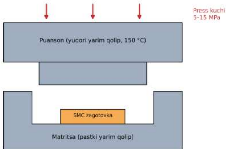
9-rasm. SMC materialini issiq presslash sxemasi
