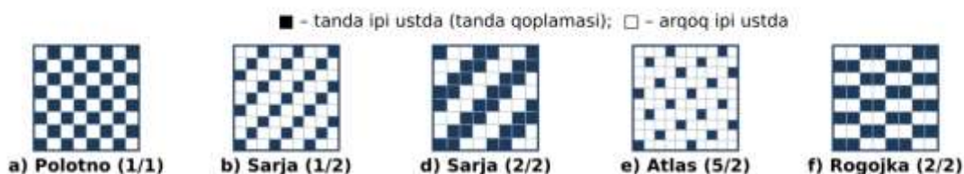
8.1-rasm. Gazlamada tanda va arqoq iplarining yo'nalishi
