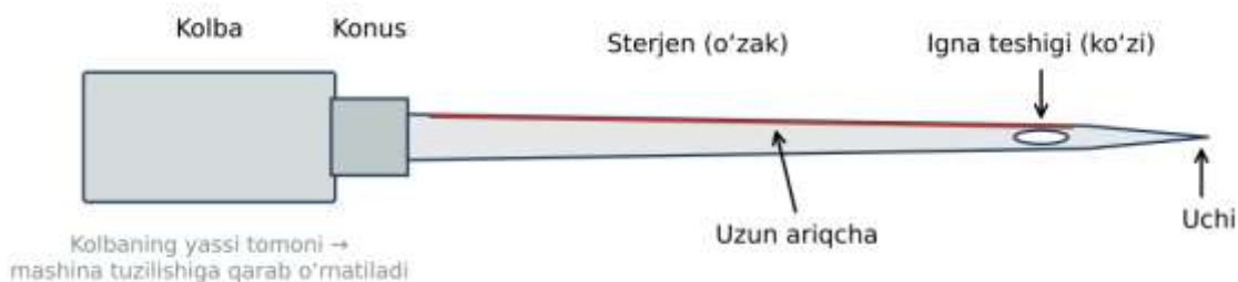
13.2-rasm. Tikuv mashinasi ignasining tuzilishi
