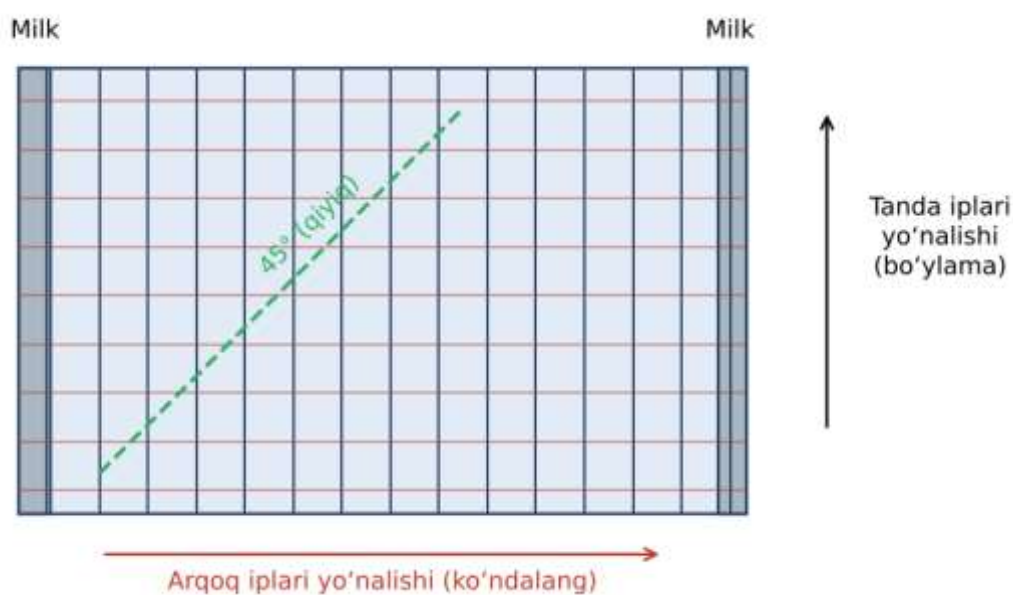
8.1-rasm. Gazlamada tanda va arqoq iplarining yo'nalishi
